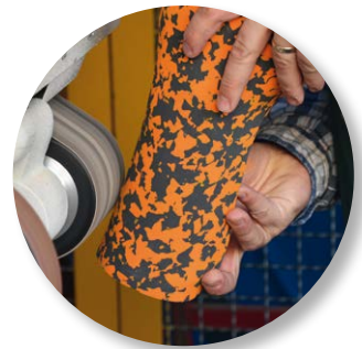
Soft socket made of Lunasoft SLW & Lunairmed
